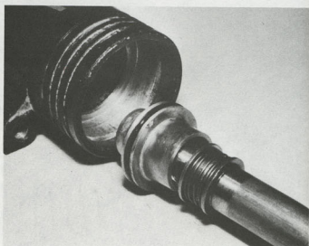
4.8b Refit damper rod assembly as shown (l.h. leg)
