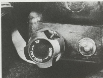
8.5a Remove screw and remove adjuster knob ...
