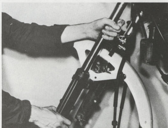
2.3d ... then pull fork legs down and clear of yokes
