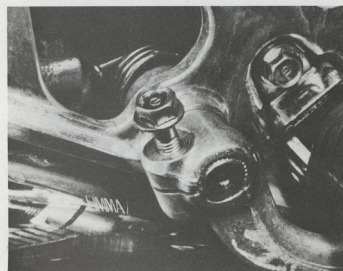
32.8c ... and brake pedal, aligning index marks
