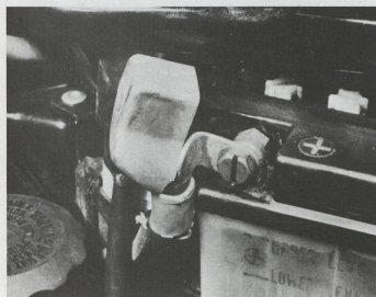
32.8a Install battery and check operation of electrical system
