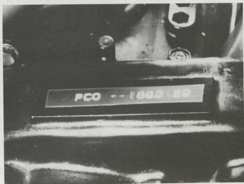
Engine number is embossed on crankcase
