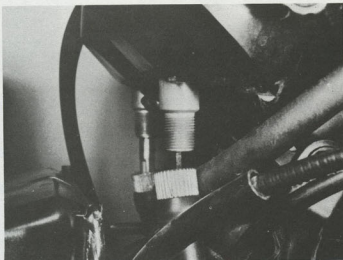
10.1a Disconnect instrument drive cables
