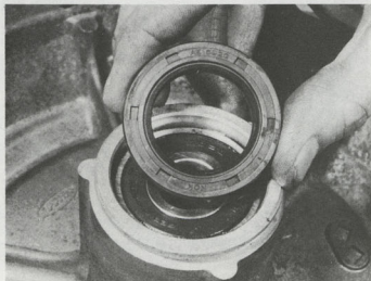
6.1d Fit grease seal to brake side of hub
