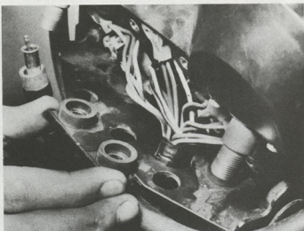
10.1b Release the panel bracket screws to free instruments
