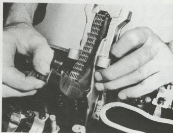
29.3b Pass chain through tensioner and fit clevis pin ...
