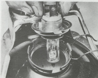
8.5f ... and lift bulb clear of headlamp reflector
