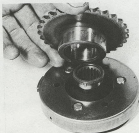
27.2b ... and install sprocket as shown
