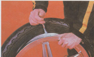
When first bead is clear, remove tyre as shown
