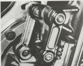
3.1b Prise off the black plastic caps which cover the screws ...
