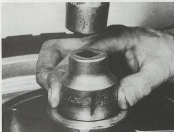
6.1c ... and drive home using large socket as drift
