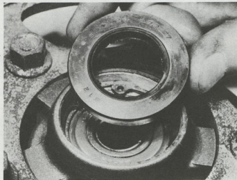
6.2b Grease seal lip and press into housing ...
