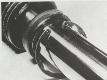
4.3b ... and remove circlip. Seal will be displaced as fork leg is removed ...
