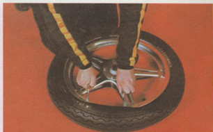
Use two levers to work bead over tyre rim
