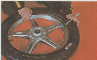
Start second bead under the rim opposite the valve
