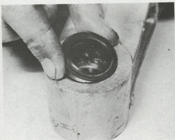
7.8a Pry out the inner grease seal ...
