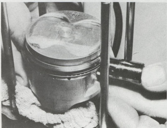
28.1a Fit pistons with 'IN' mark towards rear of crankcase
