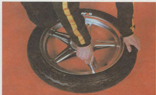
Tyre removal: Deflate tyre and insert lever in close proximity to tyre valve
