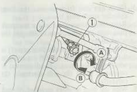
(1) Throttle stop screw (A) Increase (B) Decrease
