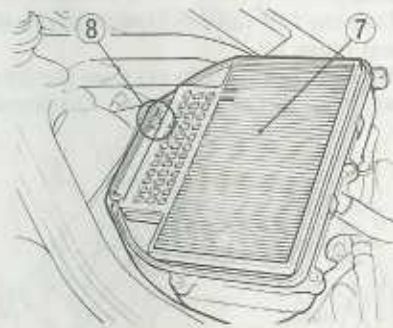
(7) Air cleaner element (8) "TOP" mark
